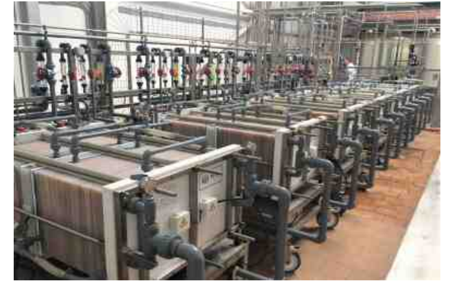
ED Plant EMU-6 for demineralization of acid and sweet whey, 24-26% TS (product quality D70). Russia, 2021
